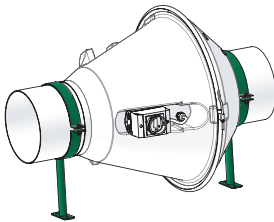
Fig. 12: Floor or ceiling mounting
